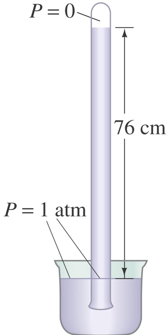
This is a mercury barometer, developed by Torricelli to measure atmospheric pressure. The height of the column of mercury is such that the pressure in the tube at the surface level is 1 atm.
